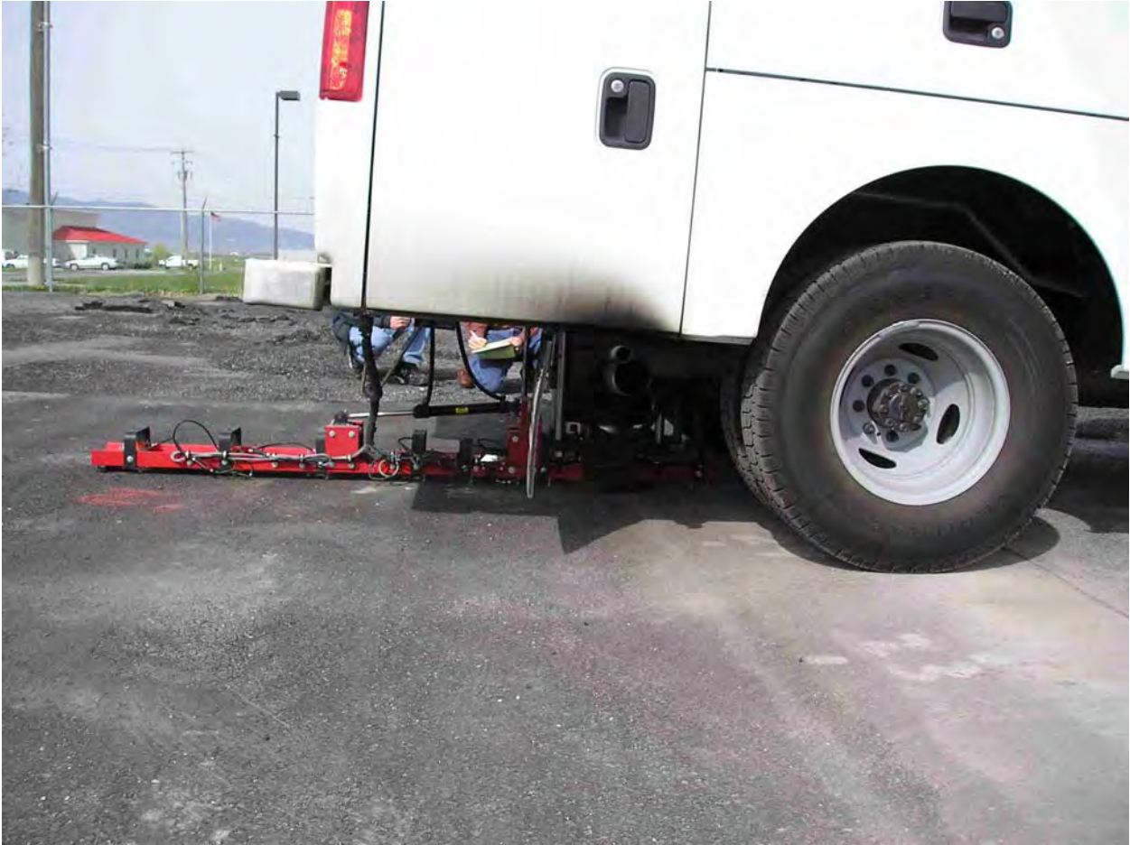
FIGURE 8 Joint evaluation with falling-weight deflectometer.
