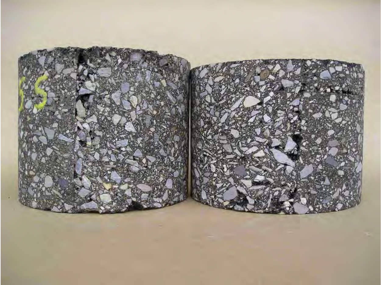
FIGURE 6 Typical cores from saw-cut joint (left) and scarified joint (right).
