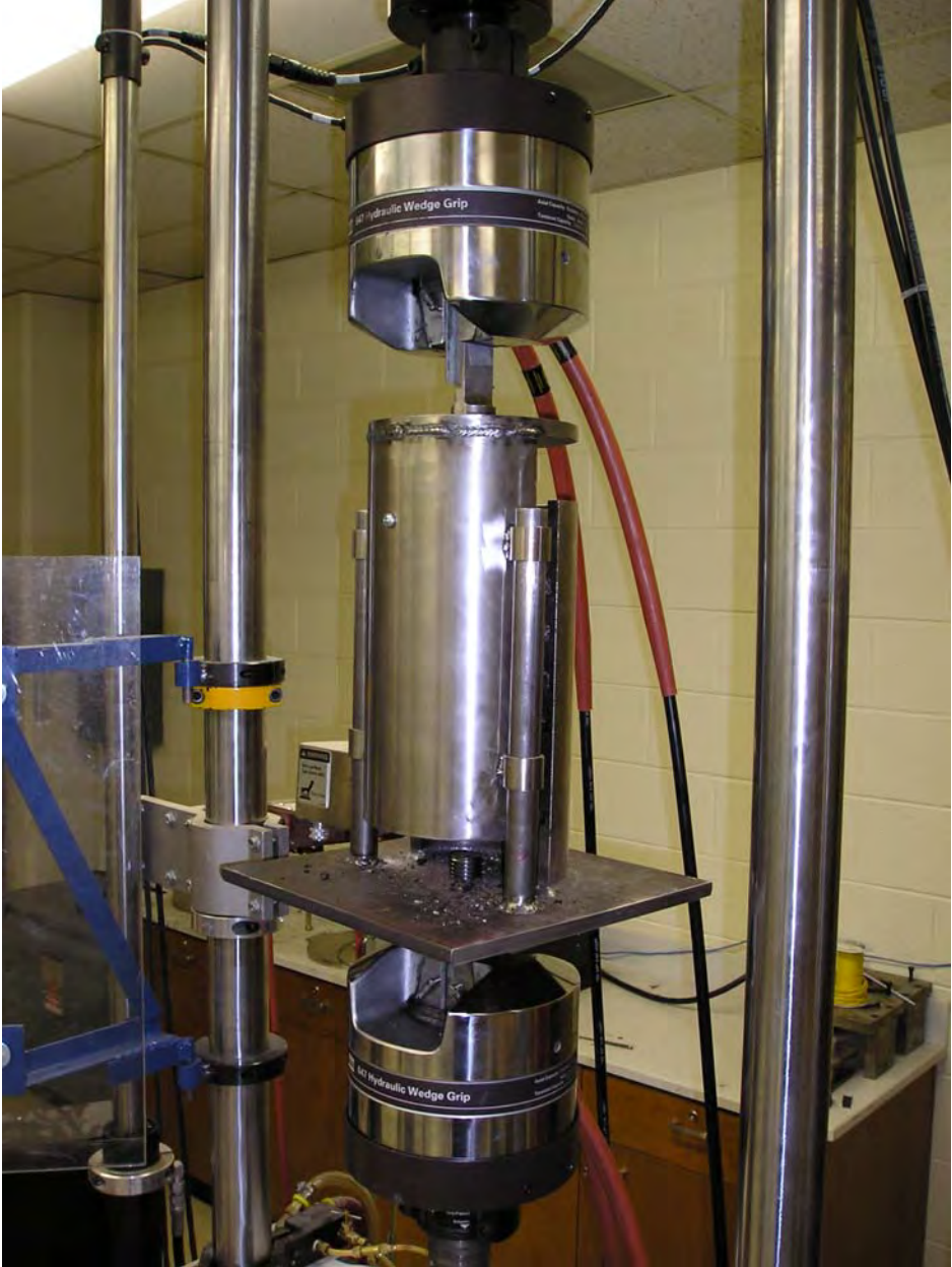
FIGURE 7 Shear testing of core specimens.
