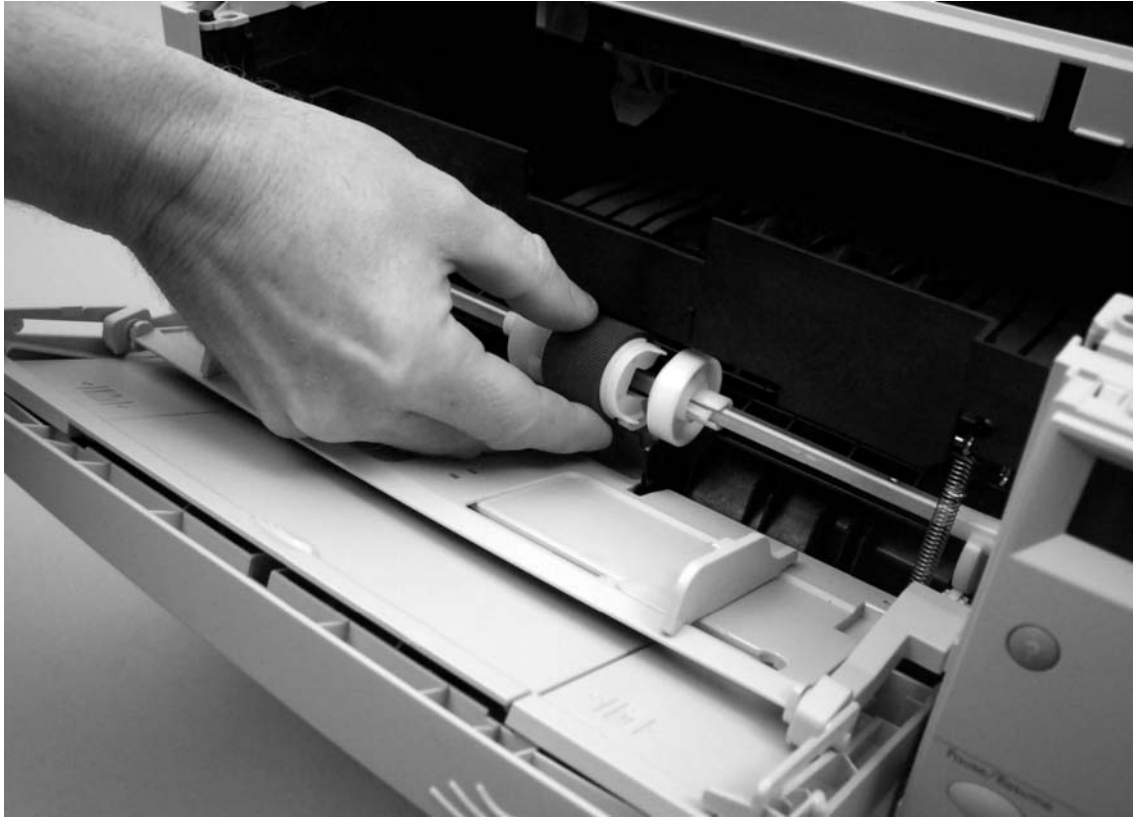
Figure 56. Removing the tray 1 pickup roller (2 of 2)
