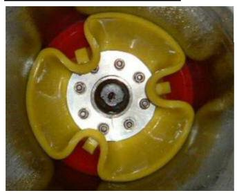
Three buckle Inducers used on SVAN project. Buckle Inducers are used to force the seals to buckle.
