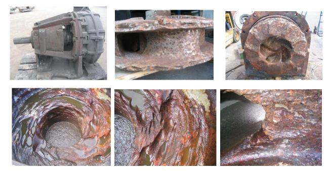
The pump unit is used for pumping slurry/fly ash product at the Power Station which is highly abrasive. The worn pump components are in excess of 500 Brinell hardness but still eroded.
