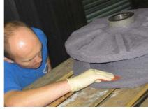
Rebuild Impeller Blade
