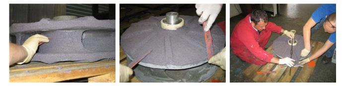
Re-build Impeller with Belzona 1121 Super XL Material
