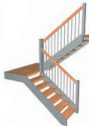
Half Turn Staircases with Landing
