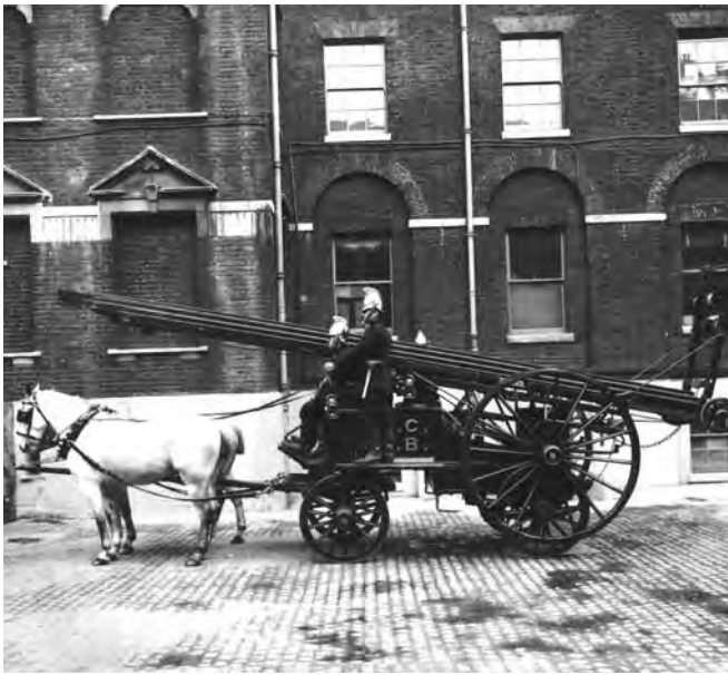
Above: A London Fire Brigade 50ft wheeled escape ladder pictured at Southwark HQ, c.1905.
