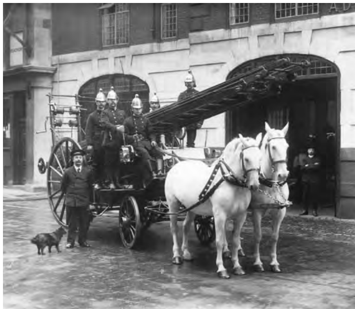
Above: A horse drawn 50ft escape ladder of the Metropolitan Fire Brigade, which became the London Fire Brigade in 1904. This view was taken c.1900 outside Redcross Street Fire Station in the Barbican area of London. Note the Superintendent and his dog and the superbly turned-out MFB horses specially bred for their strength and stamina.
