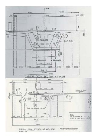
Fig. 5. Typical deck cross sections
