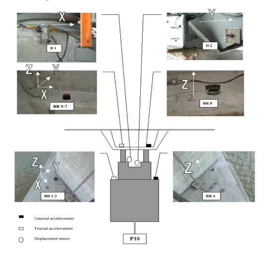
Fig. 6. Location of various accelerometer and displacement sensors at pile and pier.
