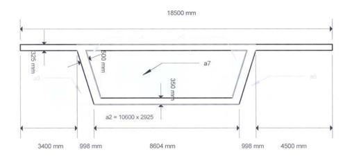
Fig. 13. Simplified deck cross-section at mid-span
