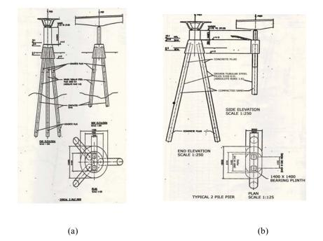
Fig. 2. General arrangement of piles (a) Three pile pier (b) Two pile pier
