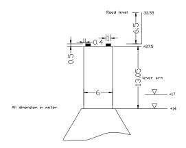
Fig. 4. Elevation of pier stem
