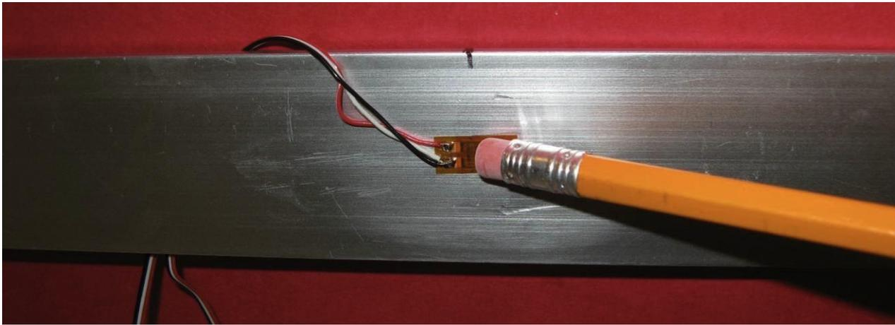
Figure 5-7 Testing the output with a rubber eraser.
