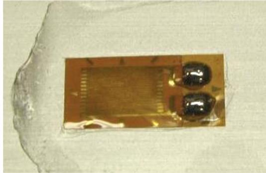
Figure 6-2: Solder bead on the two foil gage pads.
