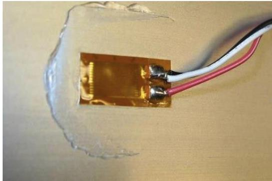
Figure 6-3: Foil gage with solder lead wires attached.
