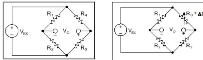
Figure 5-5 Wheatstone bridge configuration
