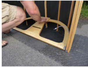
7-9. After linking the two sides, pull upwards then away from you, rotating the cross frame into place - pulling the buoyancy tubes up out of the way so they're not obstructed. The in-built buoyancy and stability tubes can now be inflated.
