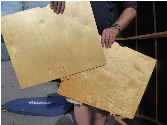
10. The two floorboards are shown here, note the difference between them. Shown here left to right are the top and bottom boards. You will see where each slots into place either side of the cross-frames, aft section (see final photo)
