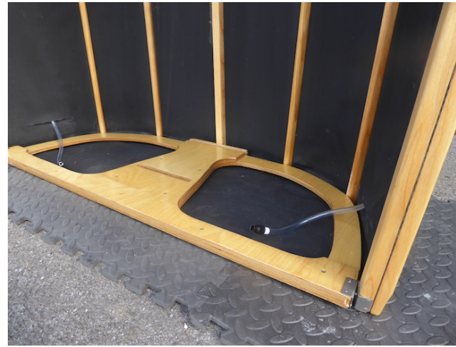
7-9. After linking the two sides, pull upwards then away from you, rotating the cross frame into place - pulling the buoyancy tubes up out of the way so they're not obstructed. The in-built buoyancy and stability tubes can now be inflated.
