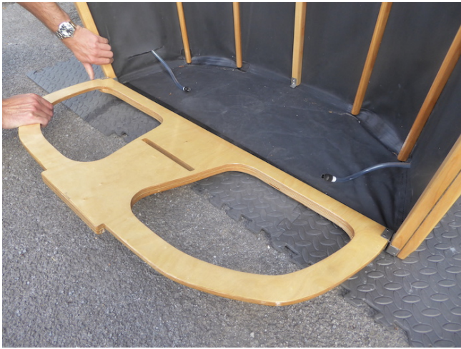
6. Repeat a similar action with the transom (aft, rear cross-frame). Be sure that the slot for the floorboard is facing downwards.
