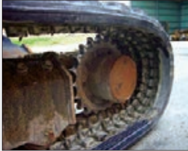
De-tracking at sprocket
