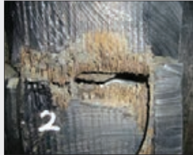
Steel cord deterioration caused by rust
