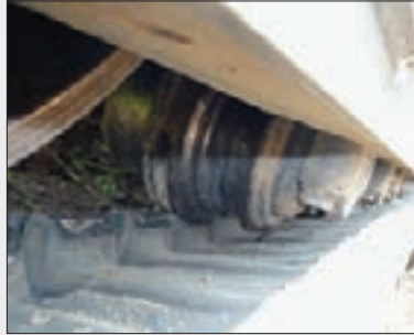
De-tracking at track roller
