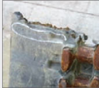
Steel cord breakage at end of overlap
