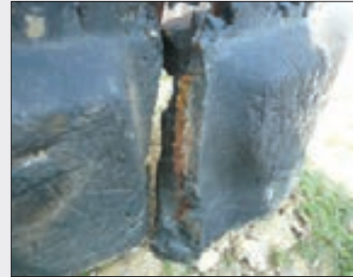
Steel cord deterioration caused by rust
