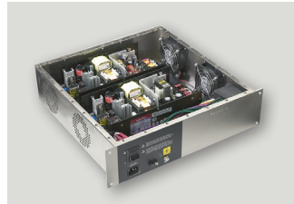
400W AC/DC open frame quad output power supply for diagnostic system.
