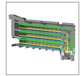
The Texas Shaker can be supplied as standard model (top loader) with access to the screens through the top of the screen box, layer by layer, and as Quick-Change (QC) model for individual access to the screen decks by opening the discharge module.
