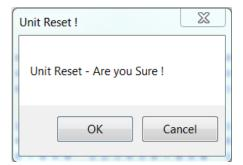
When the OK button is selected, the unit will reset and there will be no response from it. It will be about 30 seconds before communications can be re-established.
