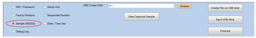
This option creates a COMMAND.TXT file which will perform the RS232 sample routine as describe in the Wi-Fi section above.
