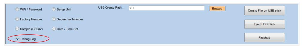
This option creates a COMMAND.TXT file which will allow the unit to write a debug log back to the USB stick.
