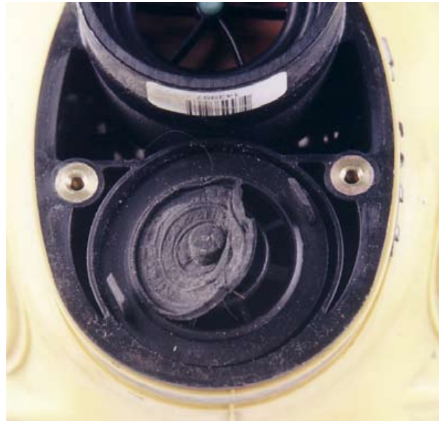
Figure 12 Badly perished and deformed exhalation valve, incapable of closing
