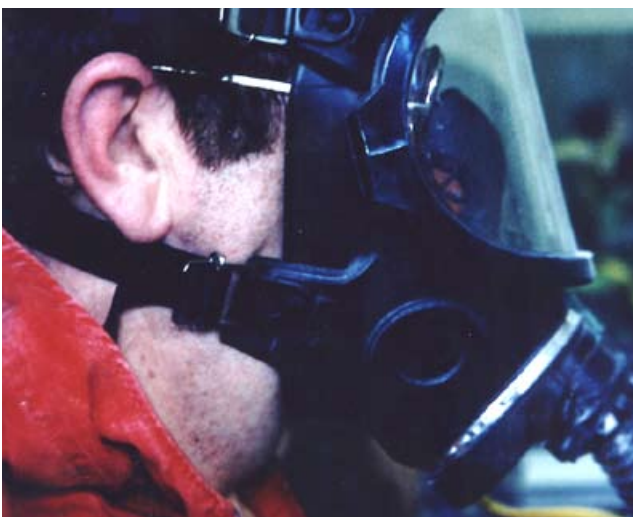
Figure 14 Ordinary side-arm spectacles worn with a full face mask, disturbing the face seal
