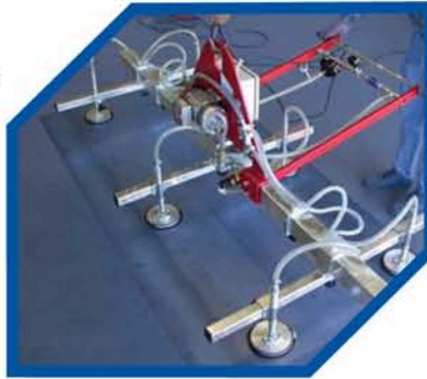
90° rotation vacuum handling granite work surfaces.
