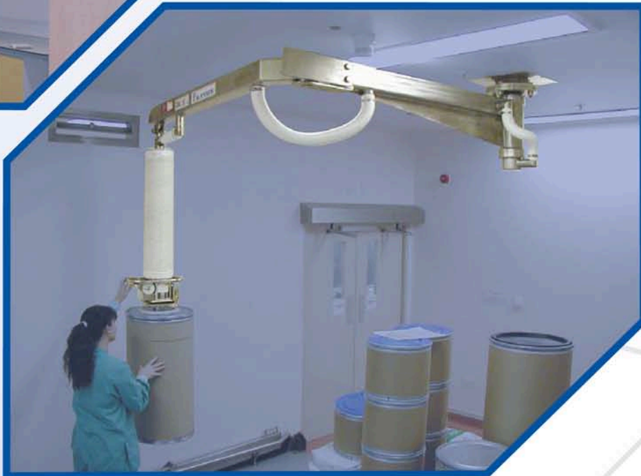
Ceiling mounted articulated arm manufactured from stainless steel.
