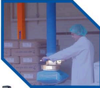
Vacuum Tube lifting suitable for sacks, worktops, drums boxes and many other products.
