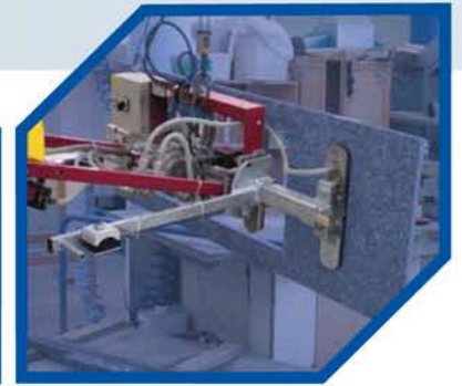
90° rotation vacuum handling granite work surfaces.
