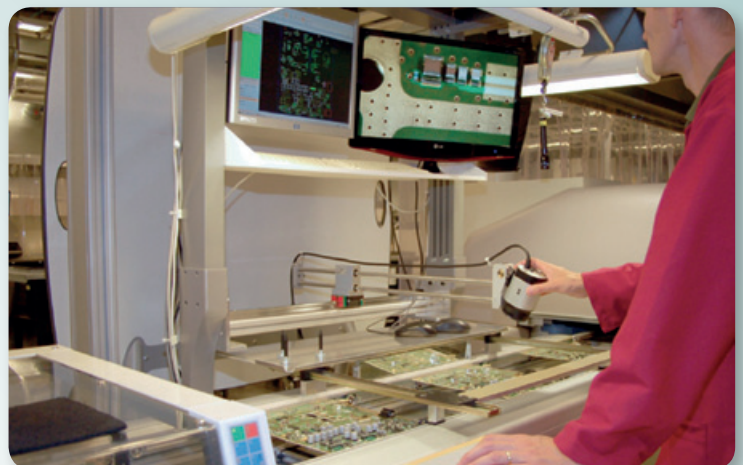
W10x-HD system with 4-directional tilt device and In-Line XY-stand mounted over conveyor in a SMT production line .
