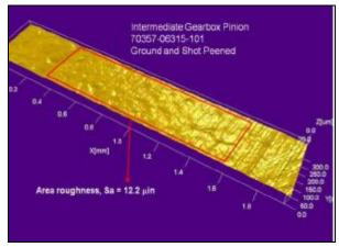
Figure 26. Surface Roughness and Topography of New Production IGB Pinion
