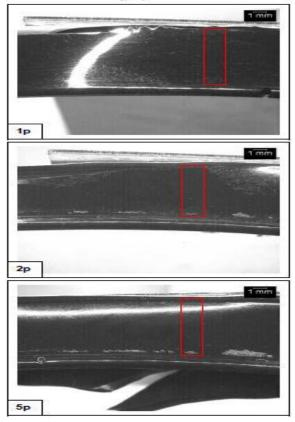
Figure 20. Replicas of TTO Pinion C518-00159 taken at 2 hrs (1p), 12.5 hrs (2p), and 33.5 hrs (5p) of test time
