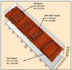
Figure 27. Surface Roughness and Topography of TTO Gear After 12.5 hrs of Testing
