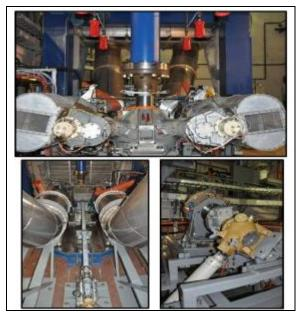
Figure18. HeDS Facility with Test Gearboxes Installed
