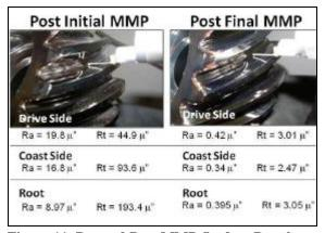
Figure 11. Pre and Post MMP Surface Roughness of TTO Bevel Pinion A518-00011
