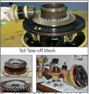
Figure 2. UH-60 Tail Drive Train Spiral Bevel Gears
