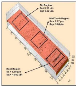
Figure 23. Surface Roughness and Topography of TTO pinion after 12.5 hrs of Testing
