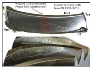
Figure 7. Silicone Replica of TTO Bevel Pinion SN A518-00011
