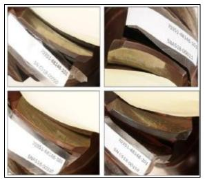
Figure 5. Driving Tooth Surfaces of Candidate Pinions
