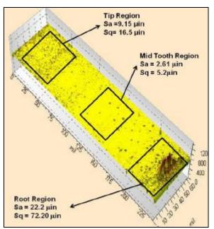
Figure 24. Surface Roughness and Topography of TTO Pinion After 33.5 hrs of Testing
