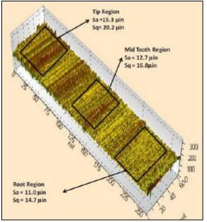
Figure 28. Surface Roughness and Topography of TTO Gear After 33.5 hrs of Testing
