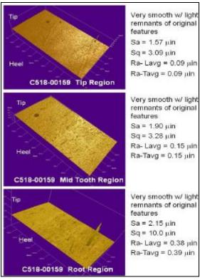
Figure 16. Pinion C518-00159 Post MMP Surface Finish and Topography Characteristics
