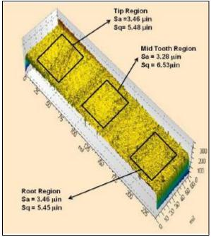
Figure 22. Surface Roughness and Topography of TTO Pinion After 2 hrs of Testing
