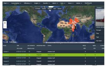
4) Remote Fuel Oil and Bunker Monitoring -Outfitting vessels with FuelTrax's Electronic Fuel Management System (EFMS) to ensure accurate fuel usage transparency and emissions tracking, to enable better fuel consumption and OPEX savings.
