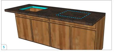
Crossville recommends cutting the Laminam after installation in order to eliminate the stresses from moving and embedding an already cut piece.
