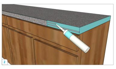
Apply wedi Joint Sealant and a strip wedi Building Panel in any thickness starting from 1/8" thick standard wedi Building Panels. This strip's cementitious coating side will allow you to better set tile.
