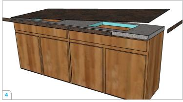
Install the Laminam over the wedi Building Panel surface and edges using a modified thinset according to section 7.1 of the Laminam Technical Manual/Guidelines found at:
