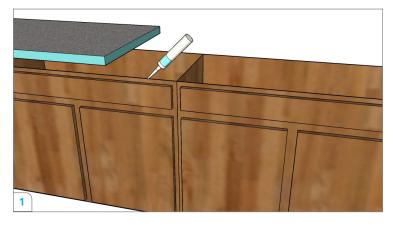
Apply a continuous 1/2" thick bead of wedi Joint Sealant over the spacers of your countertop. Glue down the wedi Building Panel in thickness of 1 1/2" to 2"after you have cut it to size. Leave it recessed behind the front of the counter so you can apply a strip of wedi Building Panel to the exposed foam edge as shown in 2 and still finish flush. Apply some weight equally on the surface for 15 minutes so that the wedi sealant/adhesive can bond properly.
