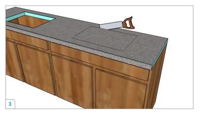
Cut out for the sink using a jigsaw or handsaw. As needed, recess cuts might be created with a utility knife or a router to accommodate recessed sinks. Cutting the holes may proceed before or after installation of Laminam as indicated in step 5.
