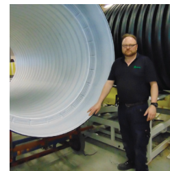
A CORMA Service Technician next to a 1400mm ID PP pipe with patented double layer in-line coupling produced on Corma's 6030 corrugator.
