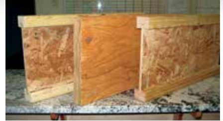
Samples of the new Preserve Tech HW preservative (Buffered Amine Oxide) for engineered wood products. Photo courtesy Royal Pacific Industries Inc.
