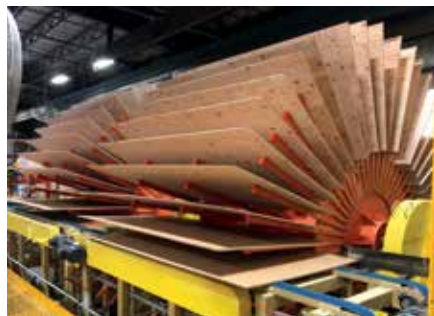
MDO in production on a 24 opening Raute press. Photo courtesy Hardel Mutual Plywood Corp.
