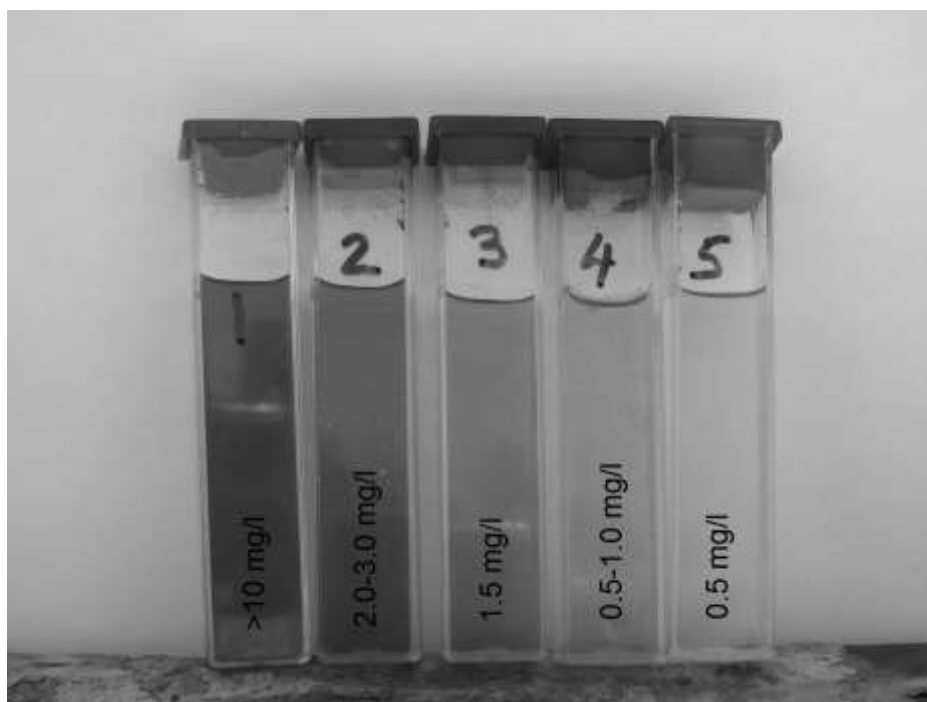
Figure 3. Results of Palintest analysis at Odengelo handpump with GI riser
