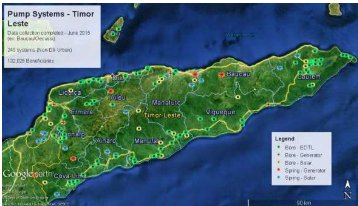
Figure 3-44: Google Earth representation of the location and types of pumped water systems in rural areas, the colour coding on the system ‘dots’ denotes the type of system and energy supply (solar/EDTL). (BESIK, 2015)
