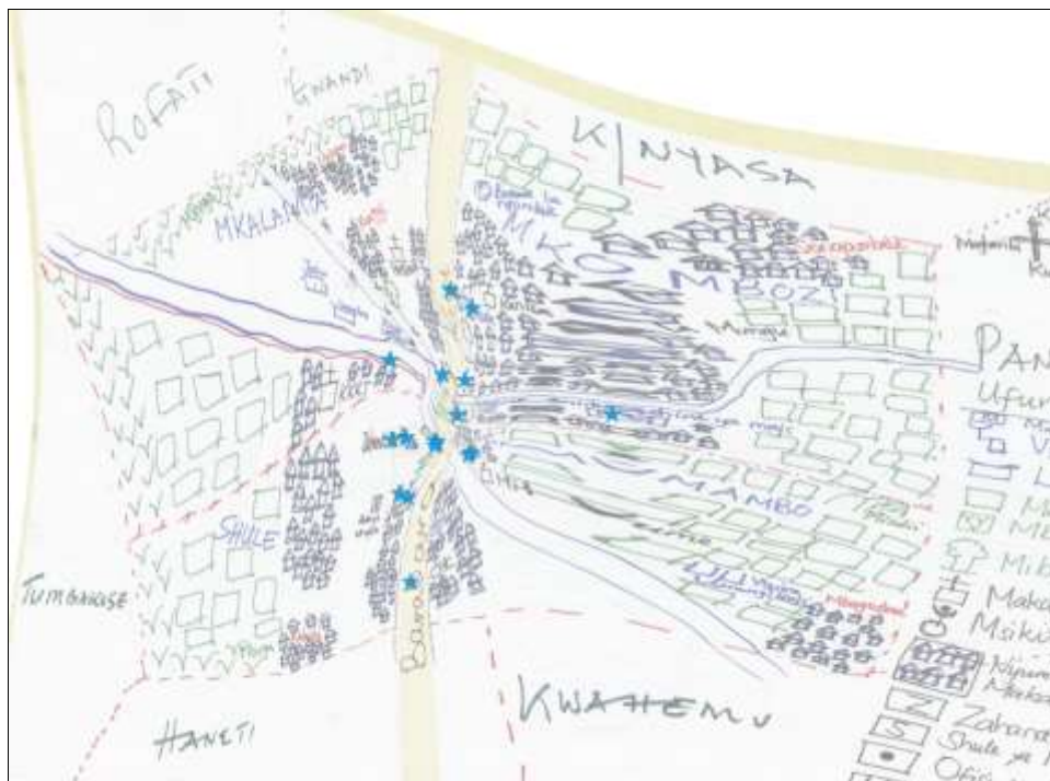
Figure 5 Distortion of Sketch map by using GPS measured locations (blue stars) as geometrical correct reference points
