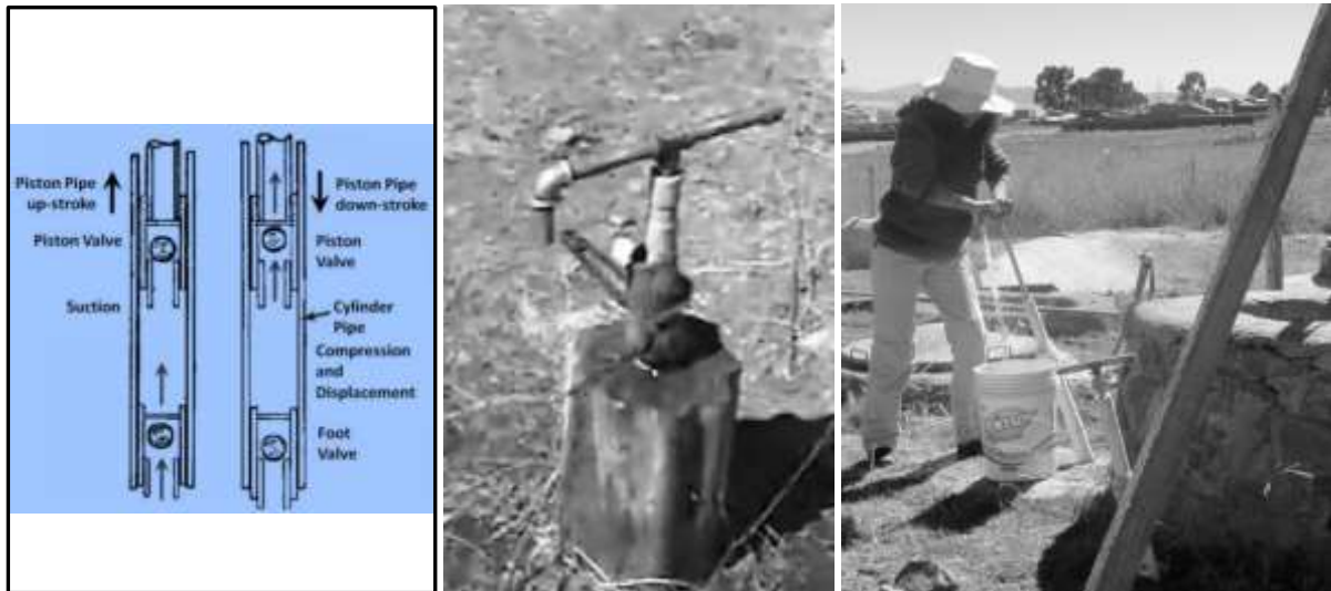
Figure 2: (a) Mode of operation of EMAS Pump: Valves function on pump upstroke [far left] and pump downstroke [left] (adapted from Buchner, 2006); EMAS Pump installed on a manually drilled well [middle, Photo: EMAS]; EMAS Pump in use, as one of several installed on a hand-dug well [right, Photo: M. MacCarthy]
