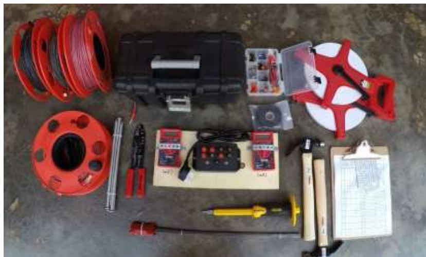
Figure 4: The Water4 resistivity toolkit consisting of control box, wire cable, spike electrodes, multimeters, measuring tapes, inverter and repair supplies.
