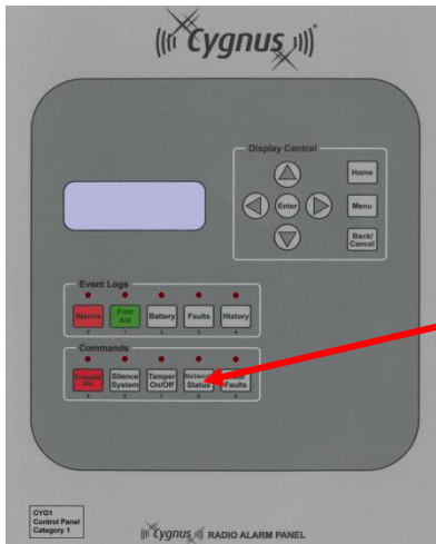
Figure 8-18: Control Panel showing the Network Status button
