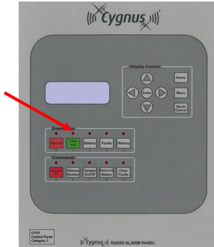
Figure 7-13: Control Panel showing the First Aid LED
