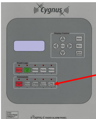
Figure 8-12: Control Panel showing the Clear Faults button
