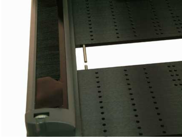
Fig. 1-3 Installation of Table Plates
