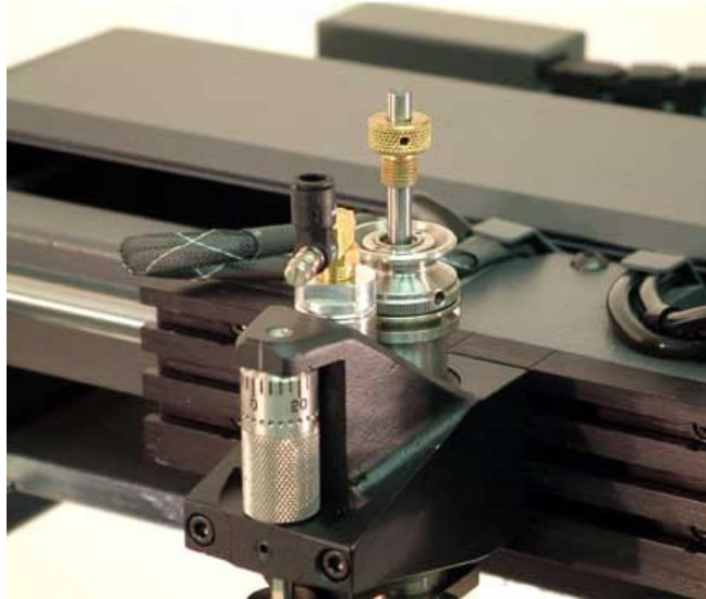
Fig. 1-28 Installation of Cutting Tool Assembly
