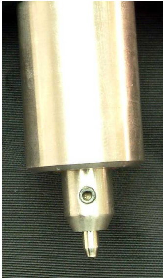
Fig. 1-25 Diamond Graver Installation
