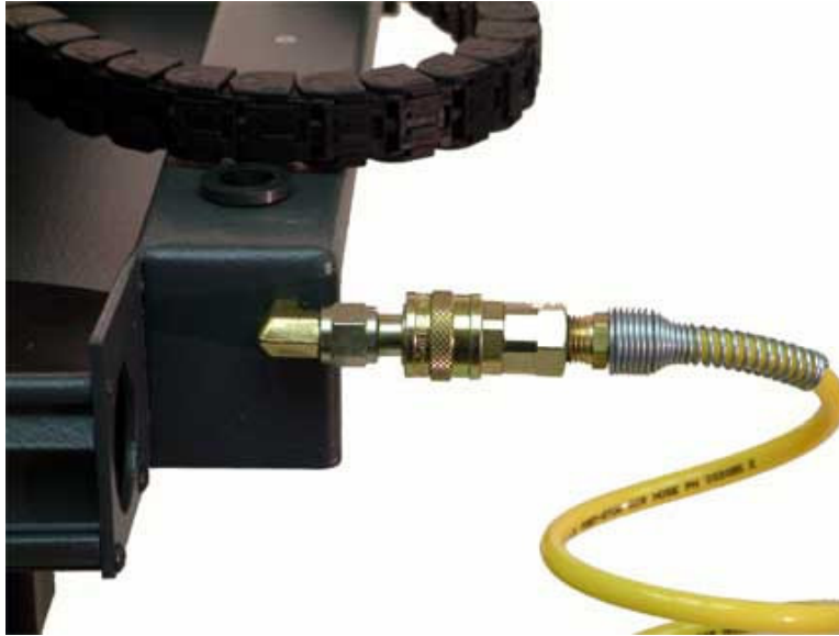
Fig. 1-17 Air Compressor Connection
