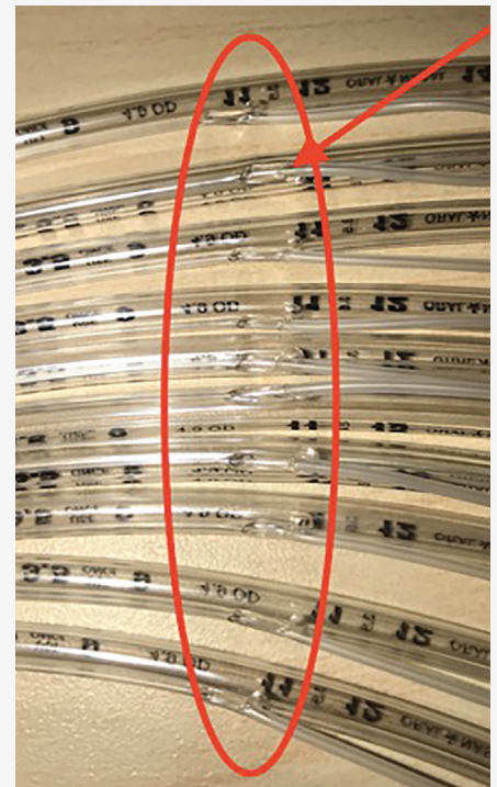
Figure 2: This figure depicts defect holes within multiple pediatric endotracheal tubes near the entrance point of the pilot balloon. The holes are of varying diameter.
