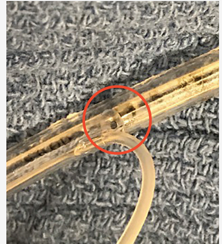
Figure 1: This figure depicts the defect hole in the pediatric endotracheal tube near the pilot balloon entrance point.
