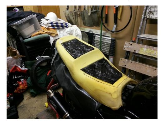
Finishing the seat was then as simple as pulling the cover back over the seat and stapling it back on.
