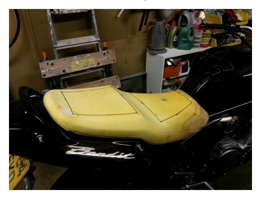
I then used a craft knife to slowly cut away the foam to about an inch in depth and to the shape drawn out on the seat,
