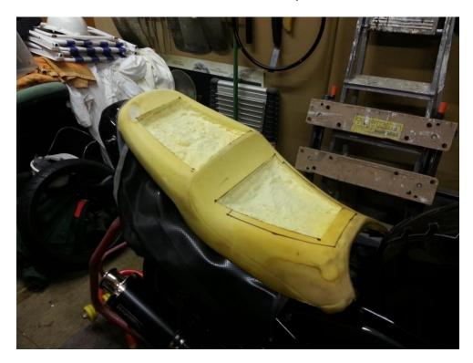
Once I had the foam cut out, I cut the gel to shape with sissors, It takes some cutting as the gel is very sticky on the inside, but holds its shape very well, just used a bit of tape to seal the edges to stop the gel sticking to everything.
