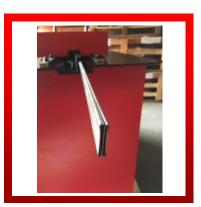
**WNS** 20swg (1.0mm) 'S' CLEAT ROLLFORMERS are 9 station machines. They are principally used in the HVAC industry for joining two ducts together in conjunction with drive cleat and plain seam rolls. Flat 'S' cleat rolls are fitted inboard with external double extended shafts, onto which many auxiliary rolls can be fitted. WNS Rollformers are manufactured with all steel side plates. The shafts, forming rolls, gears and guide fences are all hardened, and needle bearings are fitted throughout.
