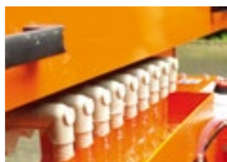
Filter outlet with drain gutter
