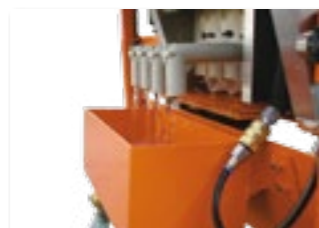
Filter outlet with drain gutter
