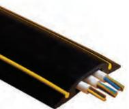
High grade fire retardant and nonconductive flexible polymer cable protector. No fixings required. Split base membrane allows cables to be pushed inside to leave the cable protector sitting flush to the floor. Gently sloping sides allow smooth passage of trucks and trolleys, whilst yellow warning stripes along each side of the profile ensures maximum visibility and reduced risk of a trip hazard.
