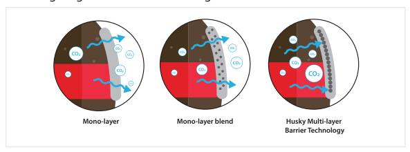
Multi-Layer Barrier packages optimize freshness by providing increased product protection.
