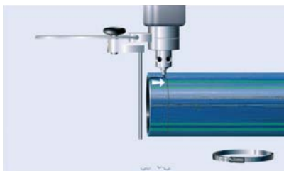
Fig 7-29: Removal of the protective coating with the egeplast coating cutter
