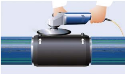
Fig 7-21: Removing the projecting wrap connectors
