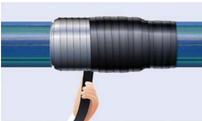
Fig 7-23: Wrapping the weld fitting with Densolen Tape AS 40
