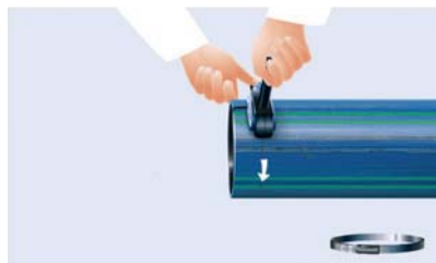
Fig 7-28: Removal of the protective coating with the egeplast M10 peeling tool
