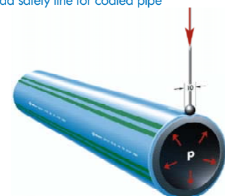
Fig 7-11: Finite element method (FEM) computational model, Muenster University of Applied Sciences, stress concentration: point and linear load safety line for coated pipe
