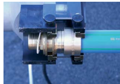
Fig 7-45: Pressing on using press tool type B
