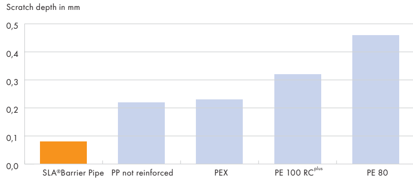
Fig 7-9: Results of scratch testing, official materials testing institute at the University of Hanover
