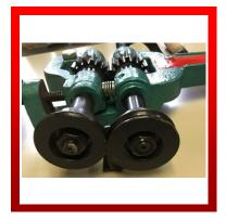
WNS HAND JENNY (HJ70-2/HJ70-4) has a 70mm throat and can accommodate mild steel up to 1.0mm thick. This machine is available with 2 Sets of Rolls which include 1 set of 7.0mm Wiring Rolls and 1 Set of Jenny rolls. OR it can be purchased with 4 Sets of Rolls which include 3.0mm & 7.0mm Wiring Rolls, 6.0mm Swage Rolls and 1 Set of Jenny Rolls.
