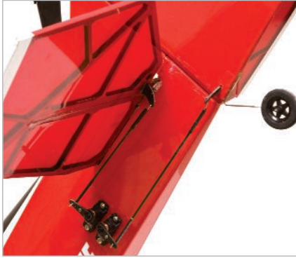
Carbon-fiber servo arm extenders and stiff pushrods promote better control response.
