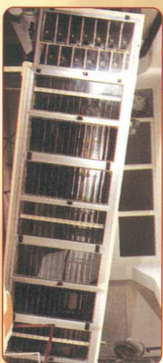
6 Belts conveyor for second proofing of the shaped disks
