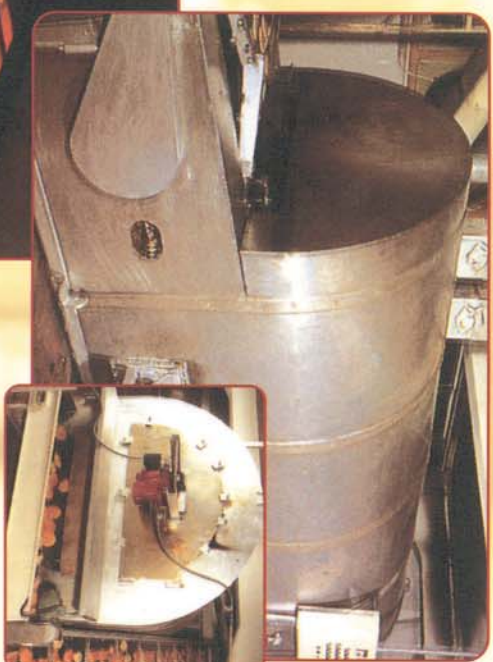
8 High temperature tunnel baking oven - heated by one gass oil burner
