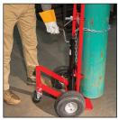
Easily raise and lower cylinder with hand crank operated jack
