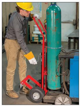
Lift-and-Load hand truck allows user to install heavy cylinders onto raised locations.
