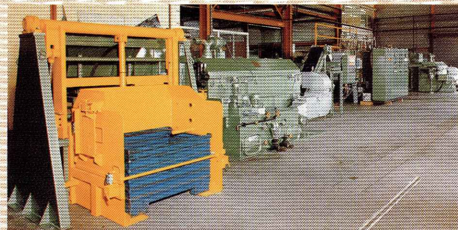
Heat treatment line with automatic loading, degreasing before and after hardening, and tempering furnace.
