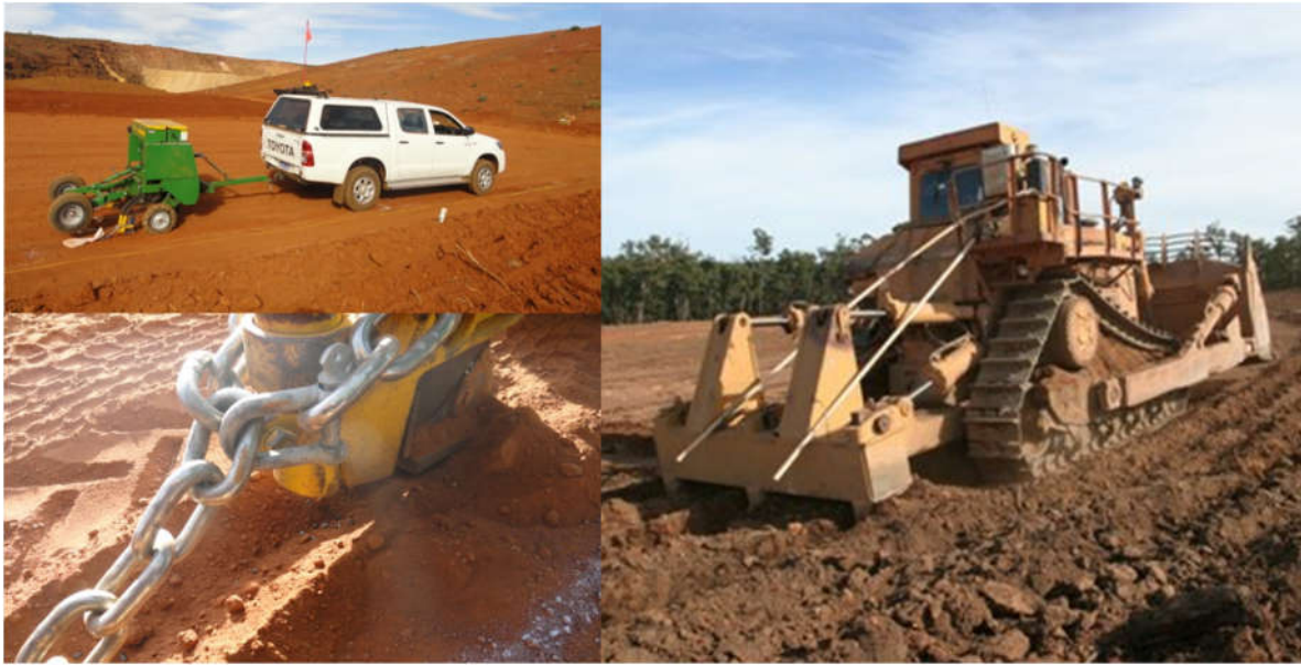
Figure 9. Seeding process with the direct seeder at Koolanooka (top left); close-up detail of the seed burial process with the direct seeder (bottom right) and an example of an air-seeder which is attached to a dozer with tines (right; courtesy of Alcoa, photo taken from http://www.alcoa.com/australia/en/info_page/mining_air_seeding.asp ).
