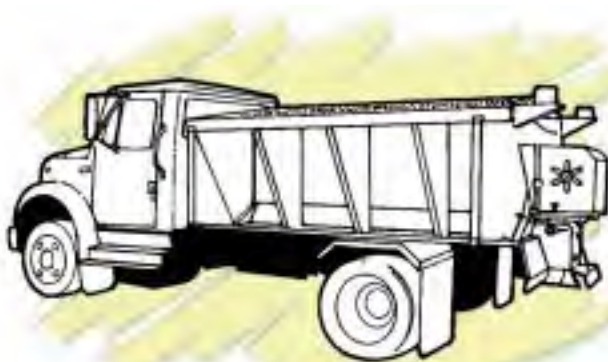
SALT AND SAND SPREADERS (A simple flip of the switch engages spreader)
