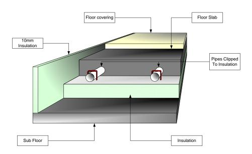
The Underfloor Heating system can be fitted in both concrete and timber suspended floors. See picture above. For other floor constructions please contact us and we will explain installation procedure, for
