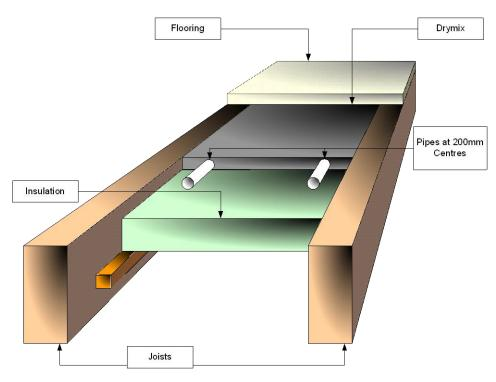
The Drymix is needed for Ground Floor, older buildings and if concrete floor and timber suspended floor are on the same floor. For First Floor applications when property is built to current building regulations an air gap is fine, still good to use the drymix as will give out more heat.
