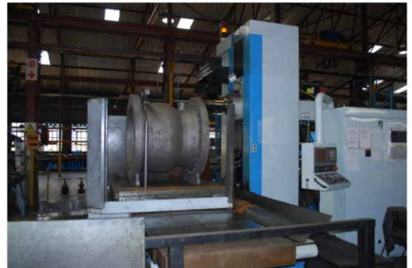
DN900 (36") PN25 NCV-B FLANGE MACHINING
