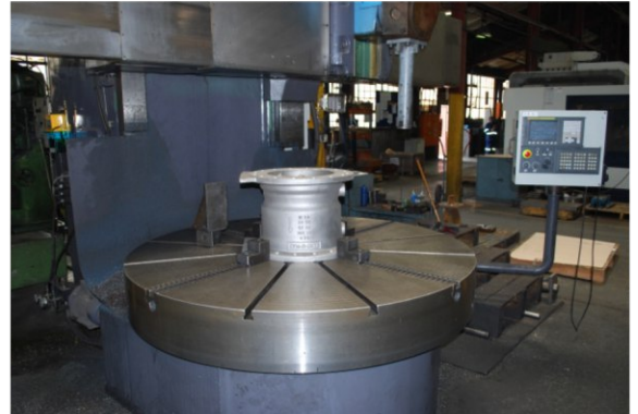
DN350 NCV-BODY SEAT MACHINING
