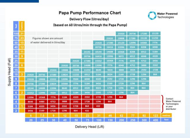
Distance pumped is dependent on delivery head and pipe friction - consult pipe manufacturer's friction chart. If more water is required, multiple pump installations can be adopted.
