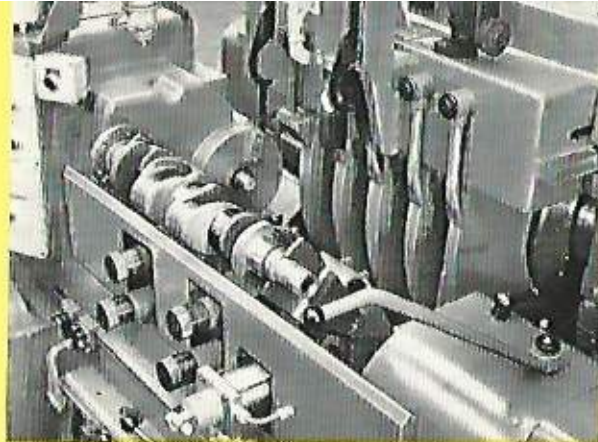
Detail of wheel assembly for machine tooled up to grind crankshaft journals. Note also the hydraulic work loader mechanism.
