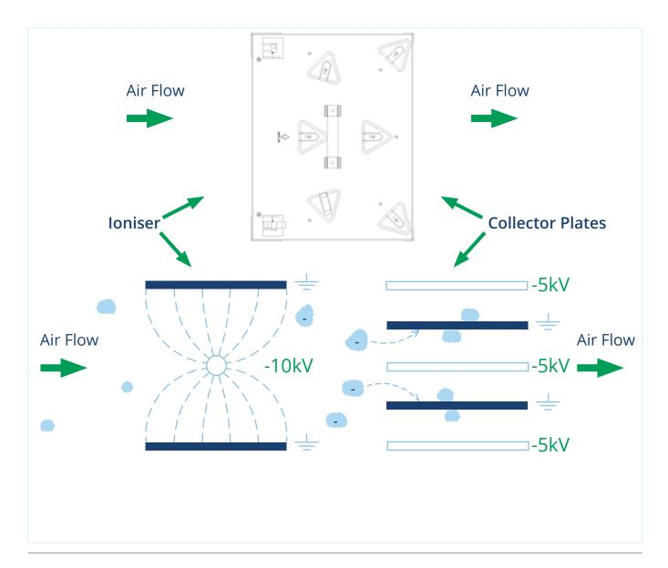
The above diagram shows, in a basic visual, how an electrostatic precipitator works. As air passes into the combined ioniser / collector cell, the particulates in the air stream are polarised to a negative potential. As they continue through the ioniser and between the collector cell plates, the polarised particulates are repelled away from the negatively charged plates and attracted to the earthed plates where they stick and so are filtered out of the air flow.
