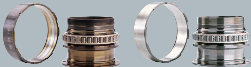
Aircraft engine bearing before (left) and after reconditioning.
