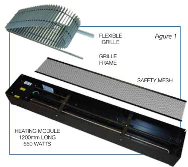
Anodised to AA15 and finished in natural satin. 70% free area on the grille and 94% free area on the safety mesh. A wide range of alternative grille finishes are available upon request. Levelling bolts are fitted through the base of the unit and provide up to 20mm vertical adjustment.
