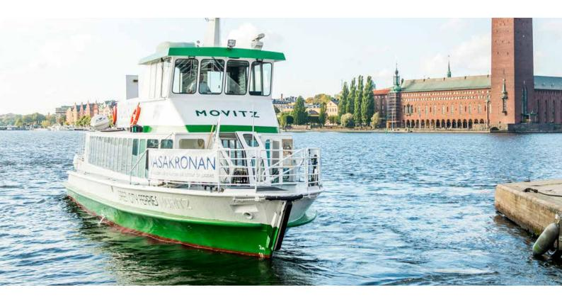
CUSTOMER: Echandia Marine INDUSTRY: Hybrid vehicle COUNTRY: Sweden ABOUT: Nilar has powered the world's first super-charged electric passenger ferry - Movitz. Its 250 kW diesel engine was replaced with a 180 kW electric and thanks to the supercharge capability of the Nilar energy storage solution, the ferry can run for 60 minutes on a single charge.
