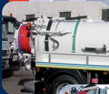
The Jet Vac Vehicle is equipped with Manual Handwheel catches with Hydraulic Door Opening and Hydraulic Tipping of the Tank. The Reel Pivots around the rear of the vehicle and is fitted with 100 metres of 19mm jetting hose with Operating Station at rear. The Rear Valves are both 4" Saunders with stack pipe on inlet with hose couplings to suit.
