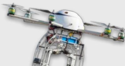
Possible extension with GoPro Hero camera, GPS USB flash drive and 2.4 GHz flight control receiver
