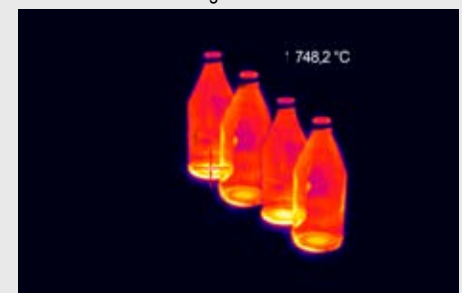
Hot-spot measurement in the production of glass bottles
