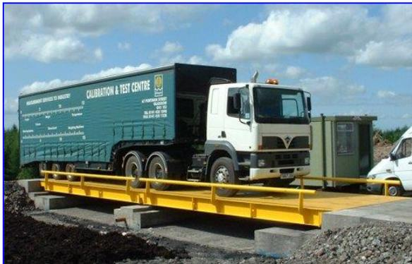
This involves the bridges being tested with calibrated weights when first installed, and then re-verified at regular periods or when any critical components are replaced. Some users insist their weighbridges are weights and measures approved even if they are not used for commercial transactions. This ensures that the weighbridges are maintained and certified for optimum precision.
