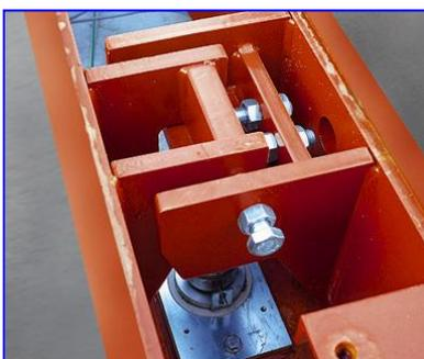
Significant end to end forces can be generated when vehicles drive on and off the weighbridge, especially if heavy braking occurs. Such forces can damage critical components such as load cells and can also cause serious damage to the surrounding structure. Effective built-in restraints are therefore an important part of any weighbridge design.
