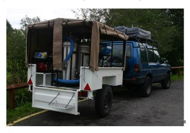
Séon UVT is equipped with multi-stage filtration, Ultra Violet disinfection, integral generator and twin self-priming pumps for full simple on site operation. Chlorine dosing is applied post filtration to ensure bacterially safe water after delivering into end user water vessels of potentially unknown sterility.
